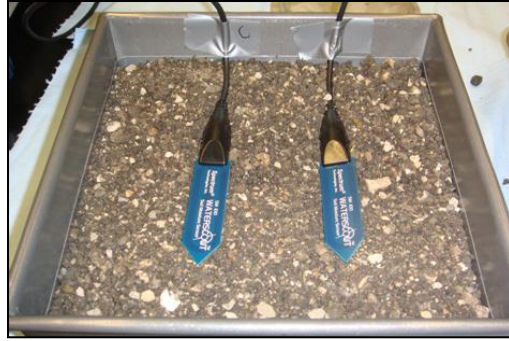
(a) Moisture sensors buried at 2.0 inches
